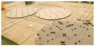
Since my initial chair designs had double curved surface the pattern had to allow for bending in more than one direction. This meant finding a pattern that has parallel overlapping cuts in at least one direction. Holes had to be distributed over the pattern to allow the sensors to 'peak trough'.
