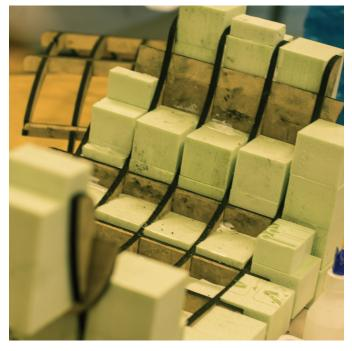
Due to the wish for - cozy - warm materials, I chose to finish the chair with felt. To provide a base for the felt the holes in the chair frame are **filled with styrodur foam**.
