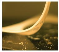
Therefore the acrylics had to be bent as well. After finding out **acrylics bend** easily at 160 degrees C, I did some trials on a stove with a huge pan for heat dispersion.
