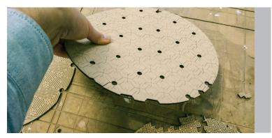
Due to limitations in wood bending I also explored a modern interpretation of the kerfing technique; **parametric laser kerf wood bending**, or lattice hinges.
