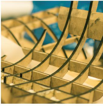
Because I refrained from the use of bent wood in the end, I needed something else to provide a rigid base with a curved shape. This is made using a **lasercut frame** for both the seating and back of the chair. This frame is made out of 8mm MDF. The holes in the frame provide room for the chair leg holders and all electronics.
